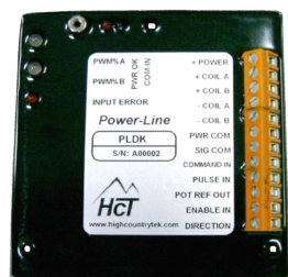
PowerLine controller shown here with standard 12 way screw terminal connector
